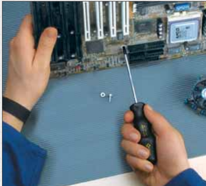
When used in conjunction with an antistatic zone, any static electricity created is discharged to ground.
