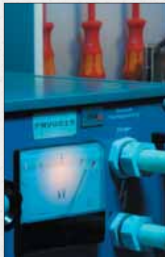
The essential quality-control inspection is the individual immersion test under 10,000 volts. This guarantees the safe performance of every single insulated tool manufactured by Wera.
