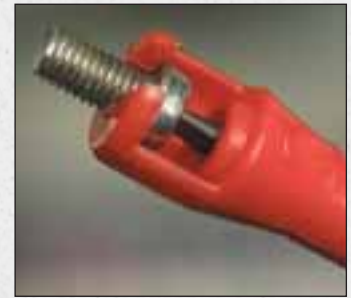
Pushing the sleeve forward makes the blades grip the screw slot, holding it securely.
